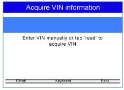
Input a valid VIN code and use the function key Finish to confirm. The scan tool starts to identify the vehicle.
