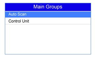
When auto scan finishes, a menu with a list of installed controllers together with their DTC overview displays.
