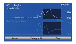
3. Press the function key **Merge Graph** to display two PID plots in one coordinate for easy and intuitive diagnosis.
