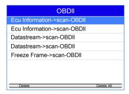
Scroll with the arrow keys to select desired testing entries and press the OK key. Details of the test record displays.
