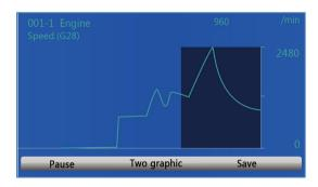
2. Press the function key **Two Graphics** to display two PID graphs in one screen.
