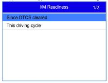
3. Depending on readiness test, one of these 2 screens will be present. Use the up and down arrow keys to scroll through data. Press the **ESC** key to exit.
