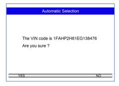
Answer YES if the Vehicle Specification or VIN code is correct and a menu of controller selection displays. Answer NO if it is incorrect, and you are required to enter the correct VIN number manually.
